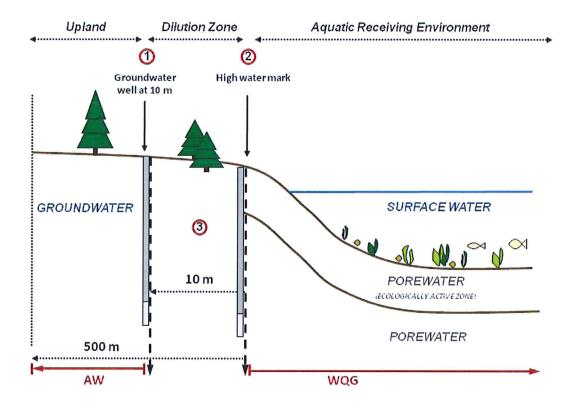
Figure 1. Illustration of the concentration limits for water in an aquatic receiving environment.
