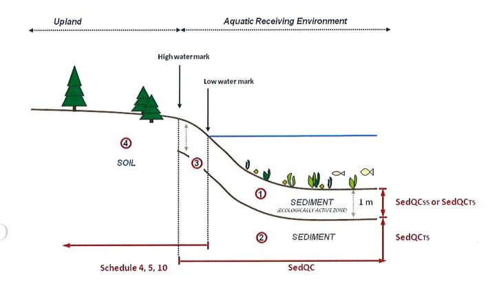
Figure 2. Illustration of the concentration limits for sediment in an aquatic receiving environment.
