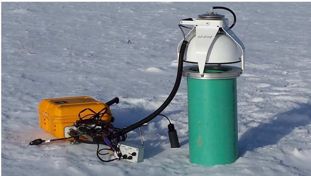
Figure C-1. LiCor System Flux Chamber and Infrared Gas Detector.
